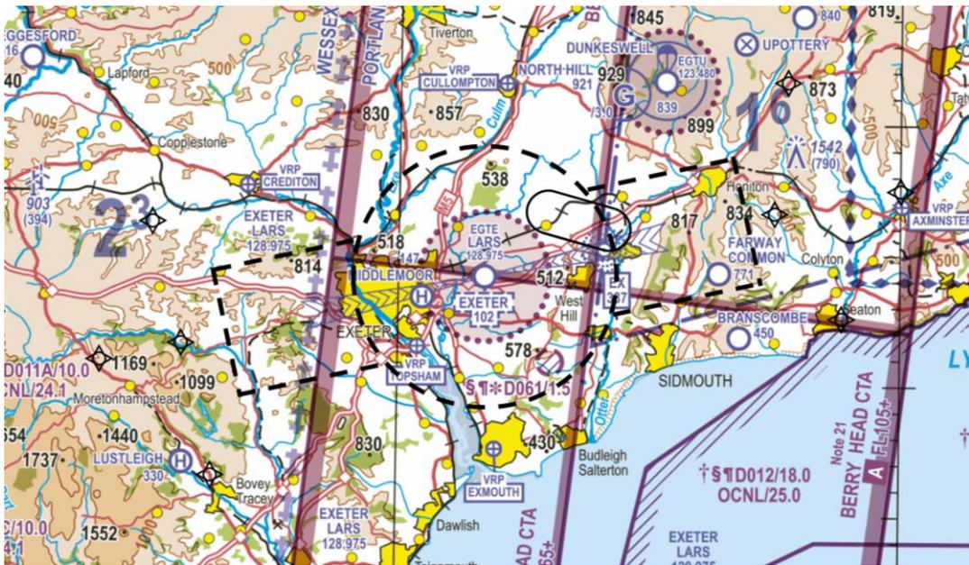
Figure 15 – 5 nm Circle with 5 nm Wide Stubs
