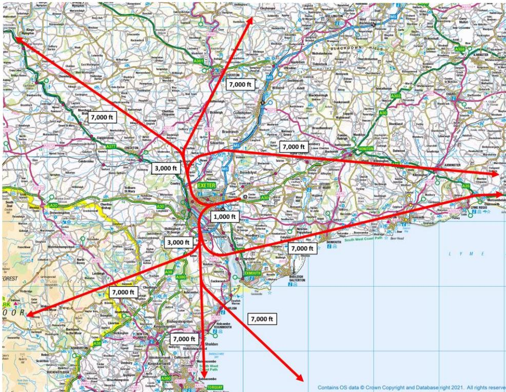
Figure 3 – Runway 26 Standard Instrument Departures (OS Mapping)
