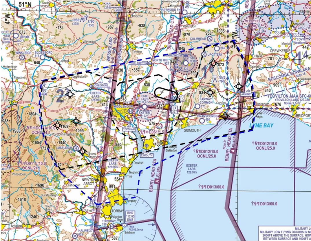
Figure 26 – 6x5 Lozenge and IAF-Protected Expanded Zone Avoiding Dunkeswell plus Upper Zone to the South
